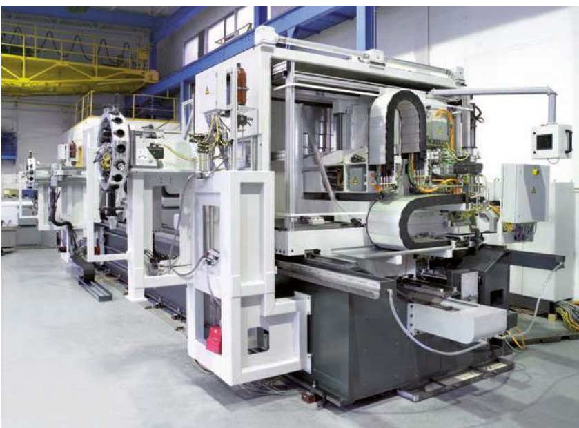
Cable carriers of the MASTER LT series on a tube end processing machine. Photographs: Rottler Werkzeugmaschinen GmbH
